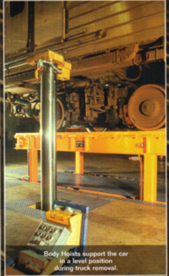
Construction is arranged so that the entire underside of the car is free of obstruction.
