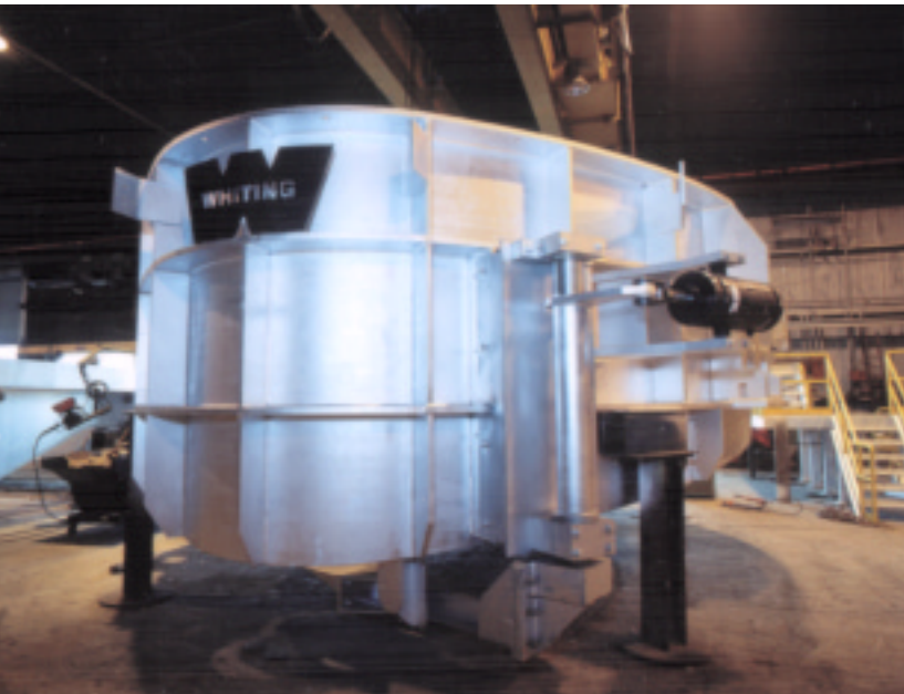
135 Ton eccentric bottom tap hearth for steel producing EAF
