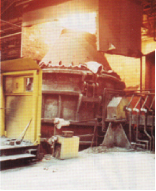
Whiting 50-ton capacity A-O-D vessel produces high-quality stainless steel.
