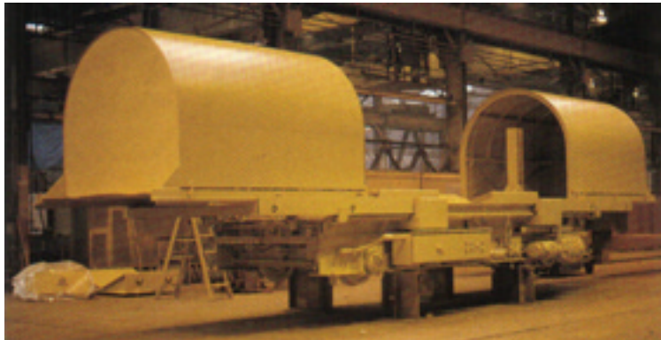
70 ton capacity, radio controlled, battery powered, steel coil transfer car with motor operated environmental protection covers.
