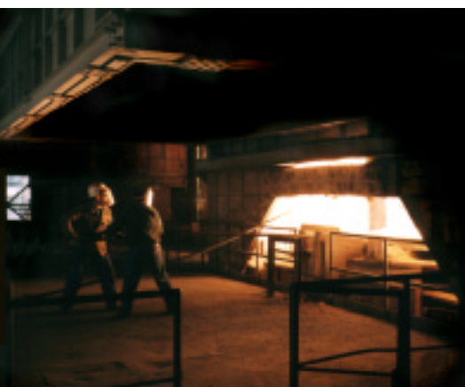
"Doghouse" style fume capture system employed on a 20 foot inner shell diameter arc furnace operation
