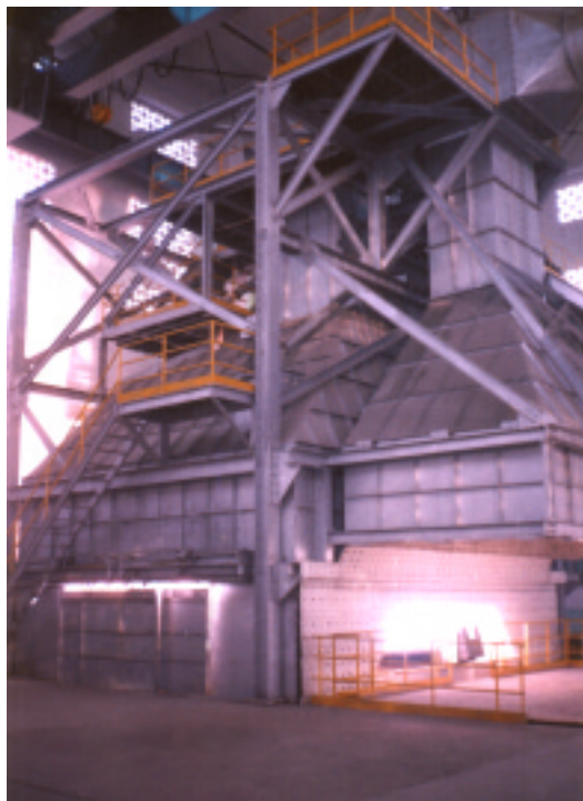
"Doghouse" style fume capture system employed on a 20 foot inner shell diameter arc furnace operation
